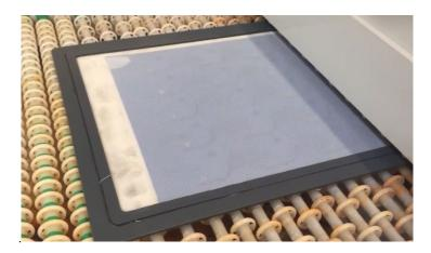
After etching is completed, remove the etched product. At this time, we will find that there is still a layer of blue film on the surface of the product.
